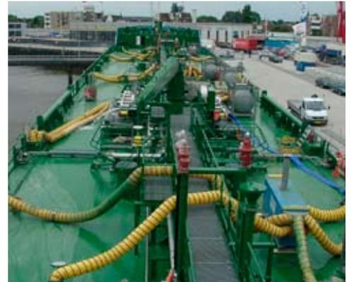
Ventilation and heating of a cargo hold.
